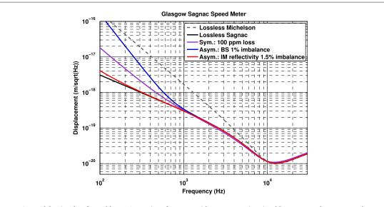
**Figure 4.** Spectral density plots for a table-top Sagnac interferometer with parameters given in table 1. Here we demonstrate what impact different imperfections have on the quantum noise sensitivity of the interferometer. All plots are drawn for phase quadrature readout, i.e. for homodyne angle  $\zeta = \pi/2$ . Ideal Michelson interferometer parameters match those of the corresponding ideal Sagnac interferometer, shown in the same plot.
