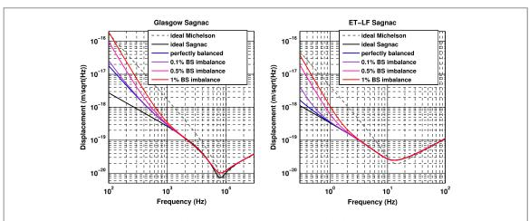
**Figure 6.** Quantum noise limited sensitivity of the Glasgow Sagnac speed meter proof-of-concept experiment (left) and a low frequency ET Sagnac interferometer (right) for an asymmetric beam splitter. Ideal Michelson interferometer parameters match those of the corresponding ideal Sagnac interferometer, shown in the same plot. (Note that all traces apart from the ones labelled 'ideal', are calculated with symmetric arm cavity losses of 25 ppm.)
