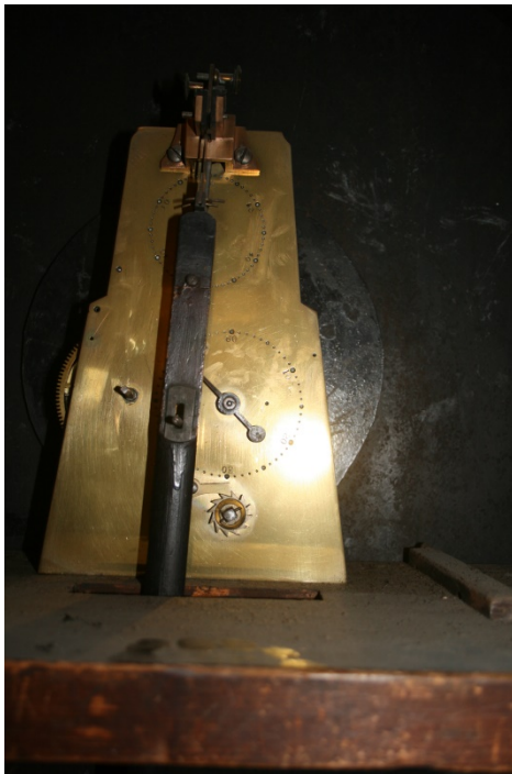
Fig. 7. The rear of the seconds' clock, originally at the the Old Glasgow College, showing a seconds' finger which is connected to a full the large sweep seconds' finger on the outer display face. The front face shows the large finger sweeping out time to the second. The mechanism and face are now housed in the West Quadrangle of Glasgow University.
