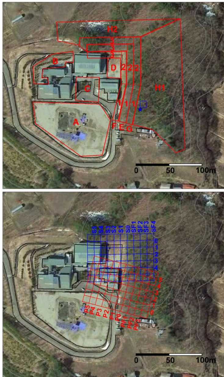
557 Figure 2. Location of survey area divisions (top), and dose rate measurement grids (bottom).
