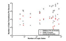
Figure: Log/Log plot of gate transitions per second for the Xilinx Simulator ISIM (on Intel i7), and the SIMD ZSIM running on both Intel i7 and Xeon Phi for circuits from IWLS suite
