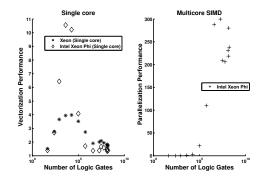
Figure: Performance comparison of single and multicore SIMD with single core sequential code on Intel Xeon Phi and Xeon. Left plot shows the speed on both machines using single core. Acceleration gain falls off for larger circuits that do not fit in 1 core's cache. Right plot shows the speedup when 240 threads SIMD where used on Intel Xeon Phi.
