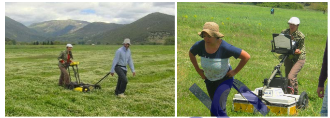
Fig. 2. Details of the employment of the single sensor Sensors and Software NOGGIN Plus-Smart Cart system with the 250 MHz antenna and the multi-channel MALÅ Imaging Radar Array (MIRA) system at the archaeological site of Mantinea.
