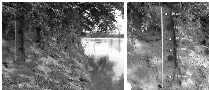
Figure 2-1: Section USU13-1, showing the distribution of the full dating and laboratory profiling samples
