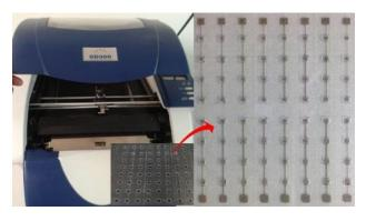
Fig. 4. 3D-Printer with developed shadow masks for nanocomposite.
