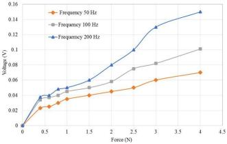
Fig. 10. Piezoelectric response of screen printed P(VDF-TrFE) sensors against different applied normal forces at various frequencies.
