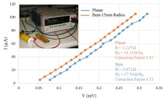
Fig. 5. Sheet resistivity in planar and bent mode (radius 25 mm) of substrate [3].
