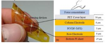
Fig. 2 (a). Optical micrograph of the whole package of 4x4 sensor array, (b). Cross sectional view of the internal structure.
