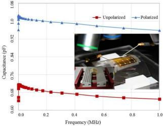
Fig. 8. Capacitance versus frequency response of printed PVDF-TrFE
