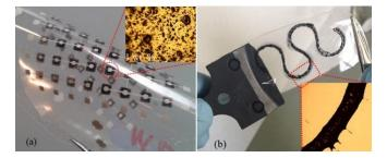
Fig. 11. (a). Printed sensors based on P(VDF-TrFE)/MWNTs on PET substrate and optical image of 1 wt.% nancomposite layer. (b) Interconnect lines of P(VDF-TrFE)-MWNTs on flexible substrate.
