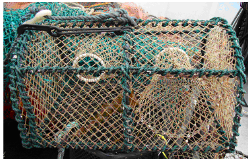
Figure 4. A Nephrops creel, showing the hard eye opening.
