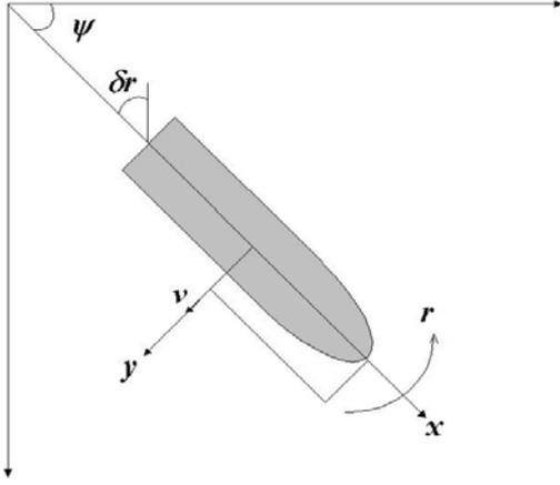
Fig 1. Notation Used to Describe Ship's Motion
