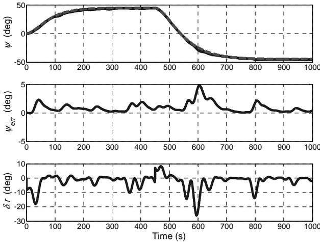
Fig 6. Cargo vessel with SM in the presence of wave disturbances.
