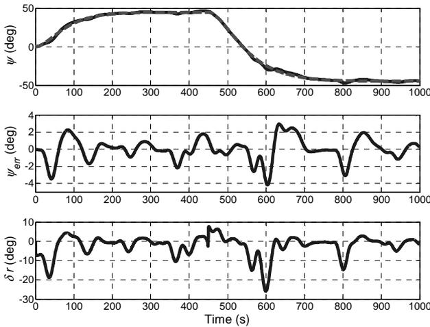
Fig 7. Cargo vessel with MPC in the presence of wave disturbances.
