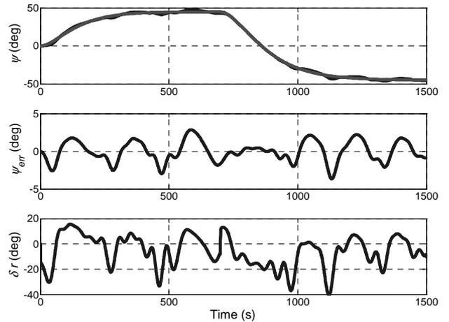
Fig 9. Oil Tanker with MPC in the presence of wave disturbances.
