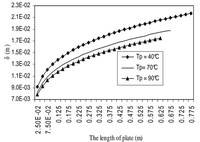
Fig 2: Thickness of the boundary layer along the vertical plate at  $T_a = 25^\circ\text{C}$ .
