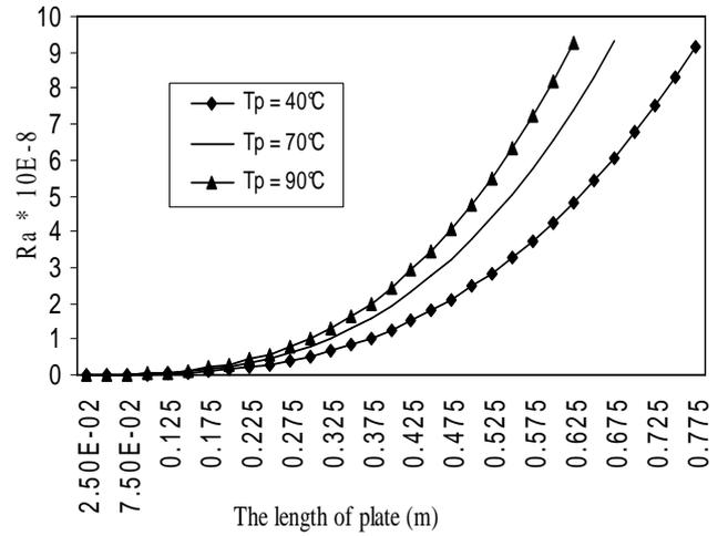
Fig 1: Rayleigh number at different location on the vertical plate at  $T_a = 25^\circ\text{C}$ .
