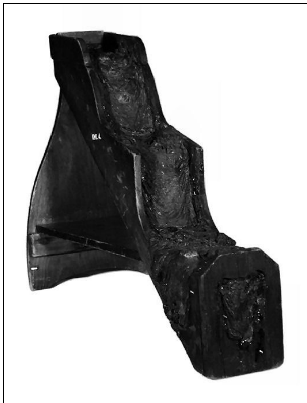
Fig. 5: Kelvin's artificial glacier experiment with pitch on a plane. Credit: © Hunterian Museum and Art Gallery, University of Glasgow.
