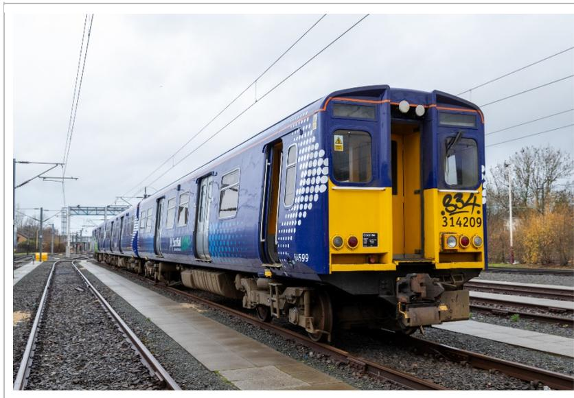
**Figure 1:** The former ScotRail Class 314 unit to be converted to hydrogen fuel-cell hybrid.
