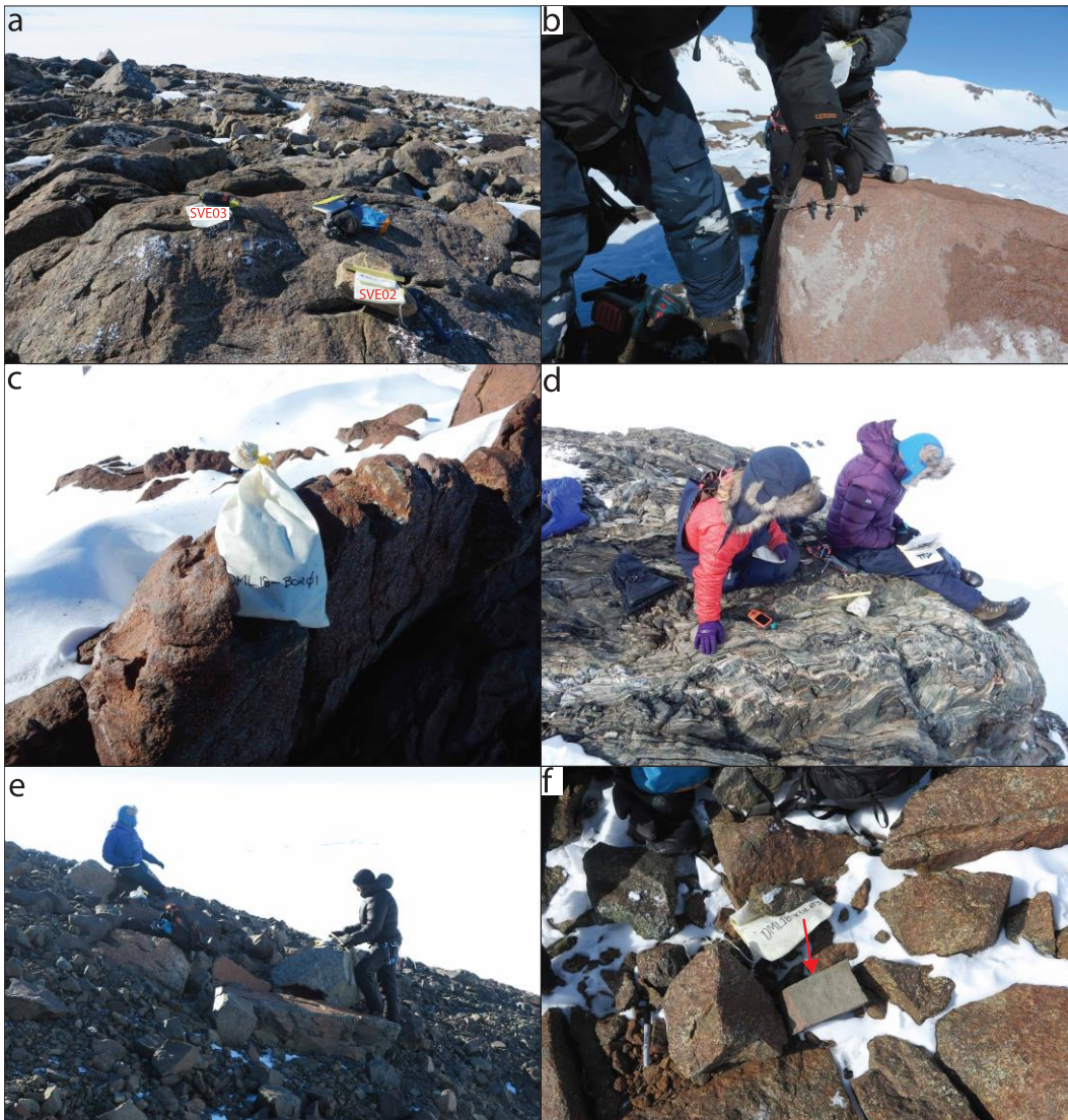
231 232 Fig. 4. Photographs of samples collected along the Penck Trough, illustrating different sample 233 types: a) the bedrock-erratic pair SVE03 and SVE02, b) GRU03, this photo also illustrates our 234 sampling method using a rock-drill, hammer and wedges, c) bedrock sample BOR01 collected from 235 ventifacted bedrock, d) MID05 erratic resting on bedrock, e) VID04 by the person to the right, note 236 that this boulder is resting on a larger slab within a slope deposit and we cannot exclude post- 237 depositional movement for this sample, and f) KUL03 (marked by red arrow) resting on bedrock. 238
