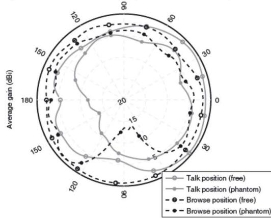
Fig 1: Pattern of smartphone antenna gain with and without a body (phantom) [3]
