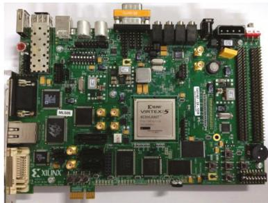
Figure 12. Xilinx ML505 field-programmable gate array (FPGA) evaluation board.
