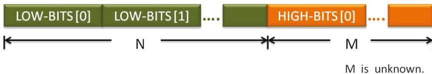
Figure 6. Fixed-block mode output format.
