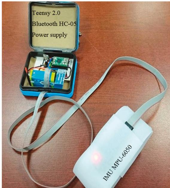
Figure 4. Portable foot attitude measuring device.
