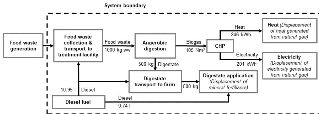
Fig. 1 System flow chart including system boundary
