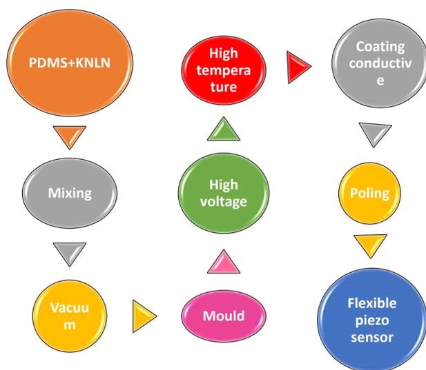
Fig2: The fabrication process of homemade piezoelectric sensors
