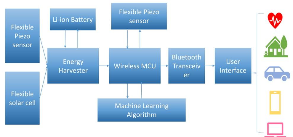
Fig1. The block diagram of smart bracelet.
