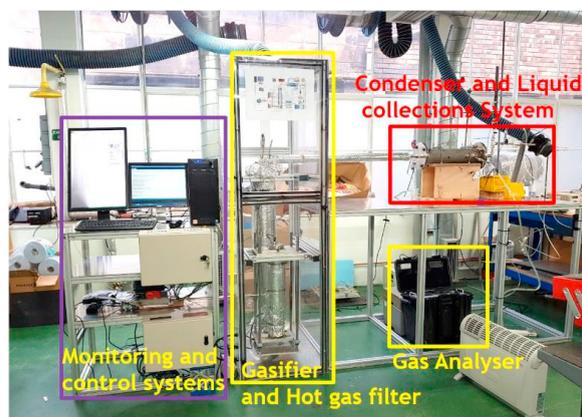
Fig. 2. Experimental setup for Glasgow's downdraft gasifier
