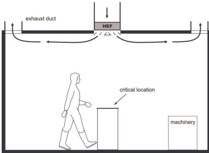
**Figure 1.** Short-circuiting of supply air in a non-UDAF cleanroom; HEF: high-efficiency filter.
