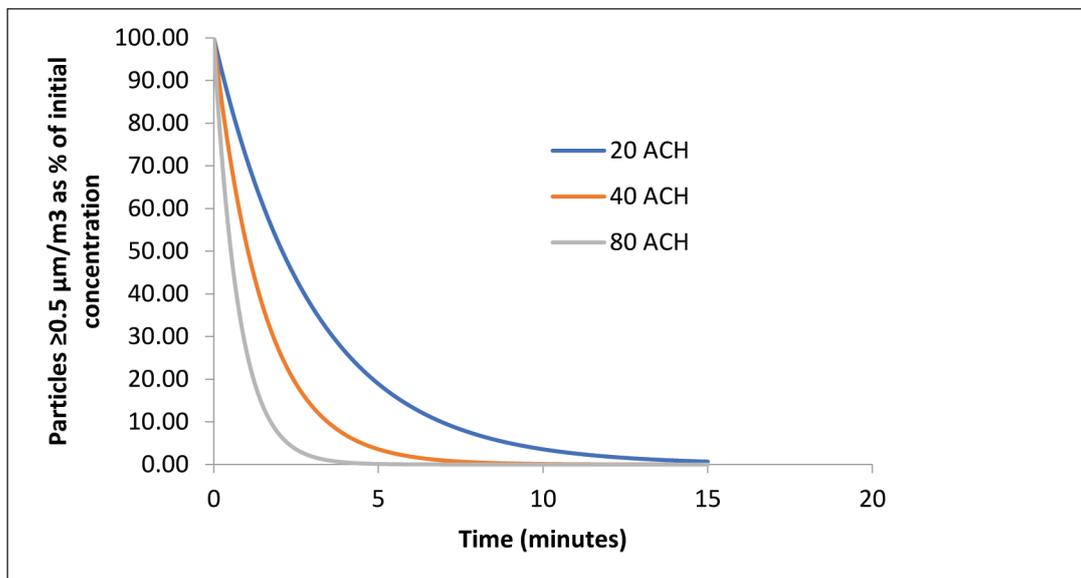
**Figure 5.** Decay of airborne particles; ACH: air changes per hour.
