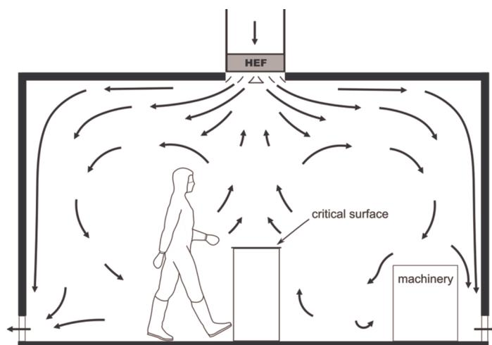
**Figure 4.** Major airflows in a non-UDAF cleanroom with a four-way diffuser at air inlet.
