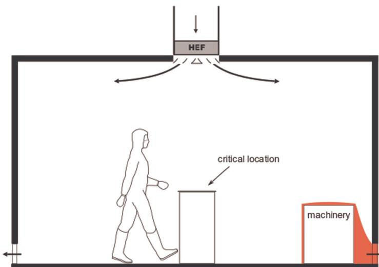
**Figure 2.** Effective removal of contaminants from machinery and high CRE index; ■ : airborne contamination.
