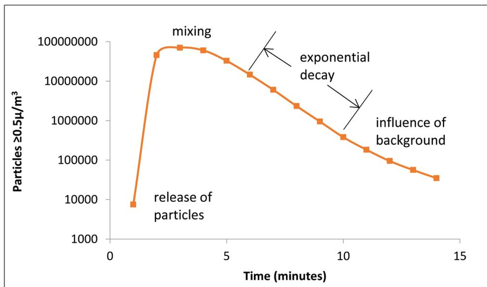
**Figure 6.** Airborne particles concentration during the recovery rate test.
