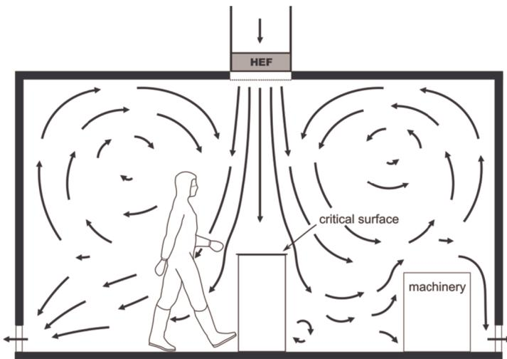
**Figure 3.** Major airflows in a non-UDAF cleanroom without an air diffuser at the air inlet.
