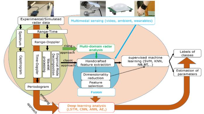
Figure 1. State of the art in radar signal processing for healthcare applications in assisted living, with conventional approach for fall detection in black color, and recent innovations highlighted in different colors.
