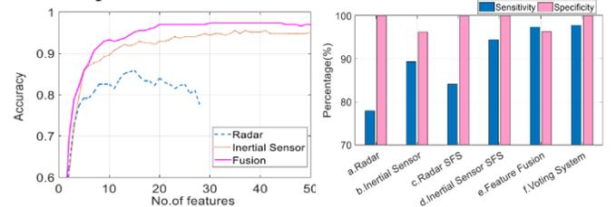
Figure 3. Classification accuracy using SFS for radar features, inertial sensor features, and feature fusion of radar + inertial data with an SVM classifier (left); sensitivity and fall specificity for different classification approaches (right) [15]
