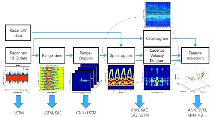
Figure 2. Typical radar signal processing chain and associated machine/deep learning method from the state of the art (SAE: stacked AutoEncoders, CAE: Convolutional AutoEncoders, LSTM: Long Short-Term Memory, CNN: Convolutional Neural Network), ANN: Artificial Neural Network.
