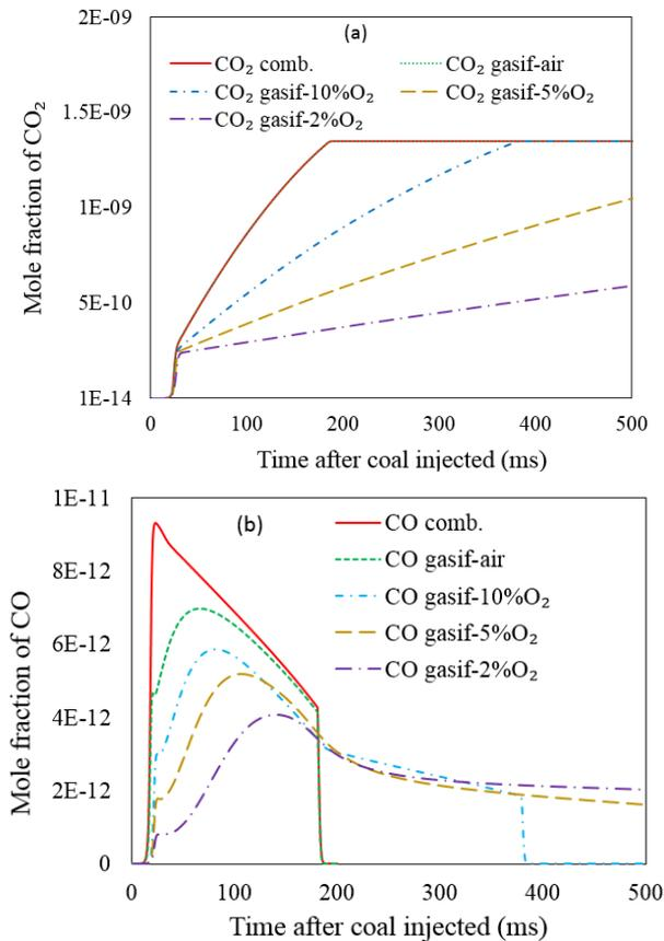
Fig. 10. The gas products under oxygen variation (a) CO<sub>2</sub> (b) CO
