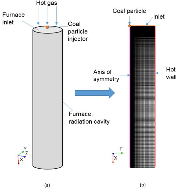
Fig. 1. An illustration of the geometry model, (a) cylindrical shape and (b) axi-symmetric model with grid
