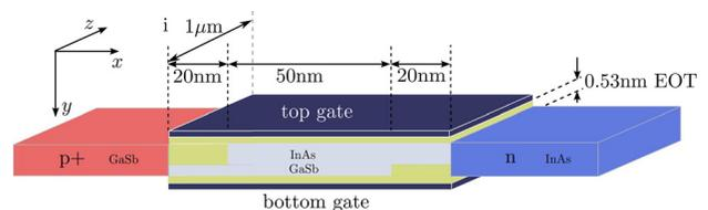
FIG. 1. Schematic representation (not to scale) of the InAs/GaSb Heterostructure EHBTFET considered in this work. Top left and bottom right HfO<sub>2</sub> spacers in the channel prevent parasitic source-to-channel and channel-to-drain BTBT from degrading the switching performance of the device.
