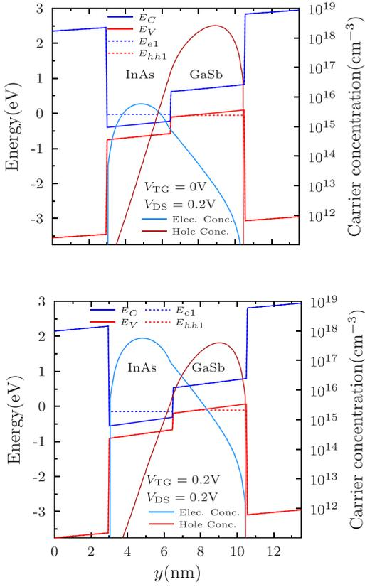
FIG. 2. Band profiles across a vertical cut taken at the center of the device for  $t_{\text{InAs}} = 3.5$  nm and  $t_{\text{GaSb}} = 4$  nm along with the corresponding quantized carrier concentrations. For  $V_{\text{TG}} = 0$  V (top), subband alignment has not been reached yet, in contrast to what happens for  $V_{\text{TG}} = 0.2$  V (bottom).
