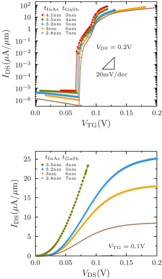
FIG. 5. (Top) Transfer characteristics of the InAs/GaSb Heterostructure EHBTFET with  $t_{\text{GaSb}} = 3, 4, 5, 6, 7\text{ nm}$ , along with the adequate selection of the InAs layer thickness inside the channel so that the  $V_{TG}$  value for the vertical BTBT onset takes place around  $0.07\text{V}$ . (Bottom) Output characteristics corresponding to  $V_{TG} = 0.1\text{V}$ .
