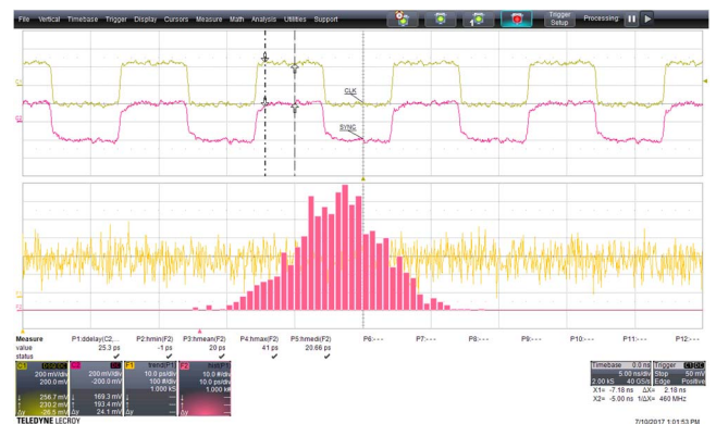
Fig. 7. Input CLK to SYNC delay after in-scope compensation.
