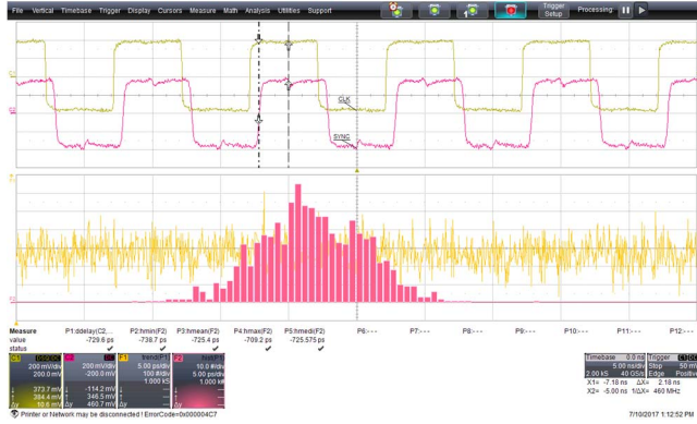
Fig. 8. CLK to SYNC delay on the backplane.
