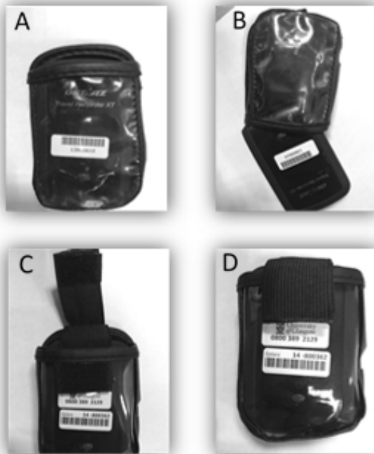
Figure 3. Demonstration of unsecure global positioning system (GPS) devices and our textile modifications to secure devices within their pouches. A: GPS device and pouch as purchased by manufacturer; B: When turned upside down or manipulated lightly the device would fall out; C: Our modification including an elasticated band and double sided Velcro attachment; and D: The additional size created was minimal resulting in a more secure pouch.
