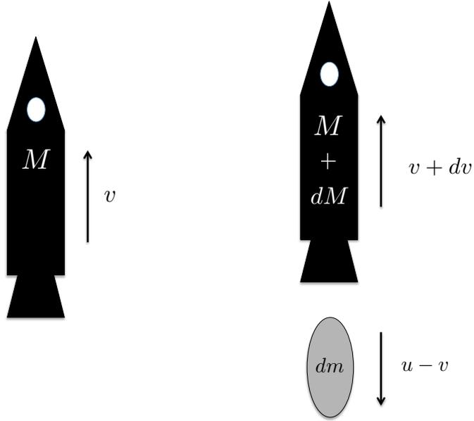
**Figure 4.** The motion of a rocket accelerated by the ejection of exhaust (adapted from Kibble's text [26]).
