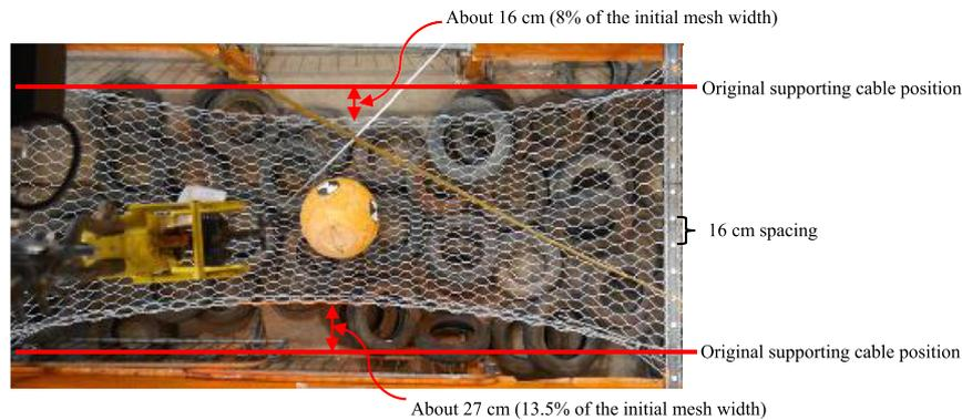
Fig. 12. Lateral deflection of the wire mesh of test 4 (top view).
