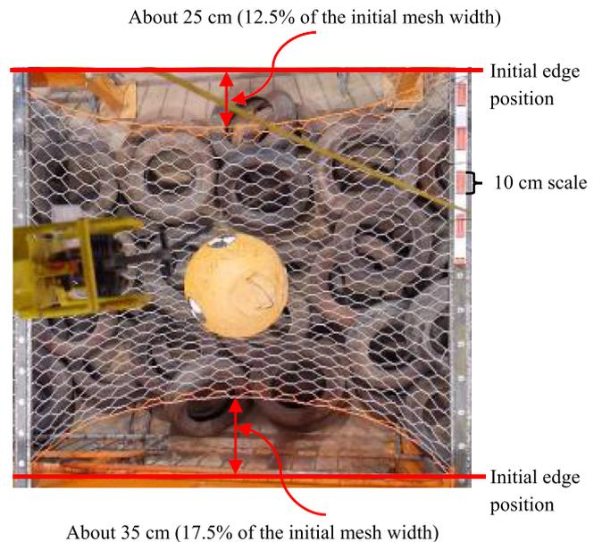
Fig. 8. Lateral deflection of the wire mesh of Test 2 (top view).
