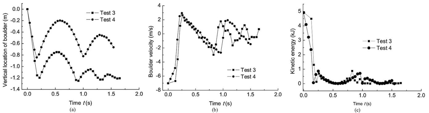
Fig. 11. Effect of the supporting cable on mesh response: (a) Vertical trajectory, (b) Vertical velocity, and (c) Kinematic energy of the boulder in Tests 3 and 4.
