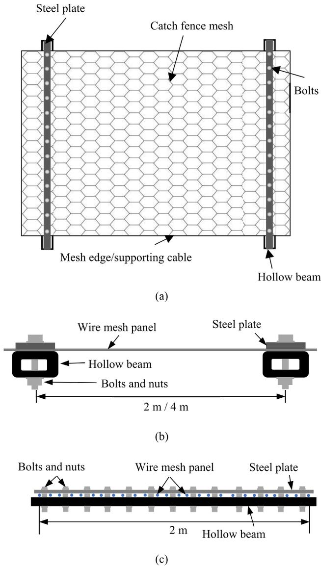
Fig. 3. Illustration of the constraint for wire mesh panels in impact tests without supporting cables: (a) Top view, (b) Front view, and (c) Side view.
