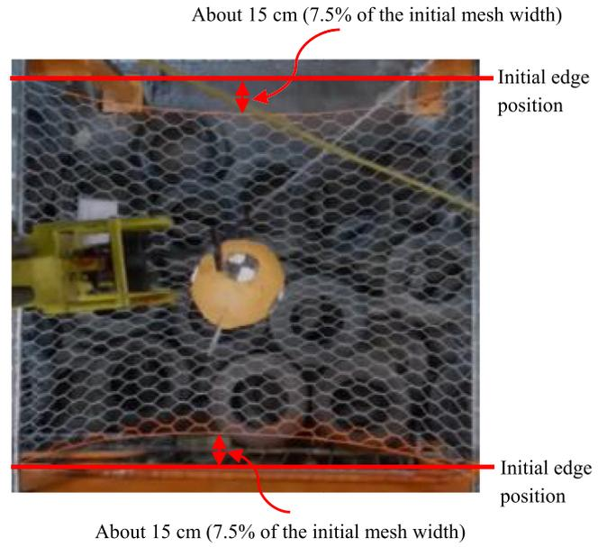
Fig. 7. Lateral deflection of the wire mesh of Test 1 (top view).
