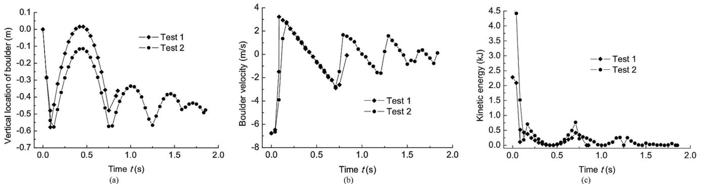
Fig. 6. Effect of the boulder size on mesh response: (a) Vertical trajectory, (b) Vertical velocity, and (c) Kinematic energy of the boulder in Tests 1 and 2.
