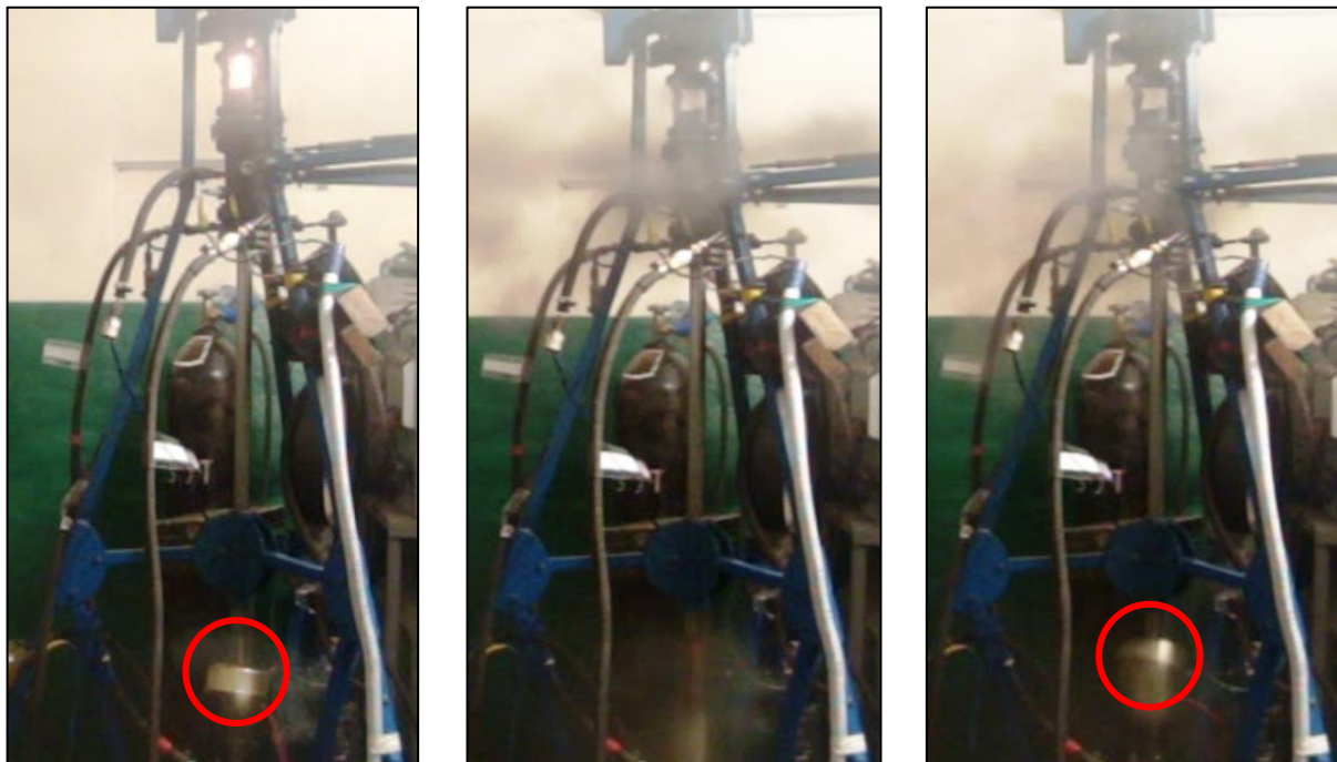
Fig. 9 An explosive failure. Forced deflection of the ram and force transducer cover (circled) may be seen.
