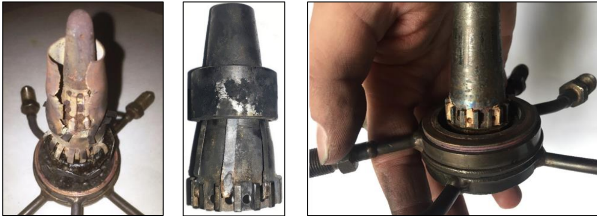
Fig. 8 Engines disassembled after burns which ended in failure (left and middle) and fuel exhaustion (right).
