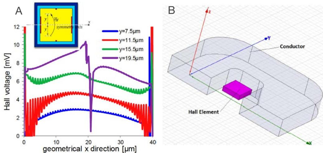
Figure 9. (A) Simulation Hall voltage along  $x$  direction for a  $40 \mu\text{m} \times 40 \mu\text{m}$  sensor and (B) Simulation Model.(Crescentini et al. 2017)
