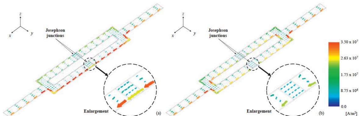
Figure 12. Current density distribution on (A) Superconducting state and (B) Voltage state.
