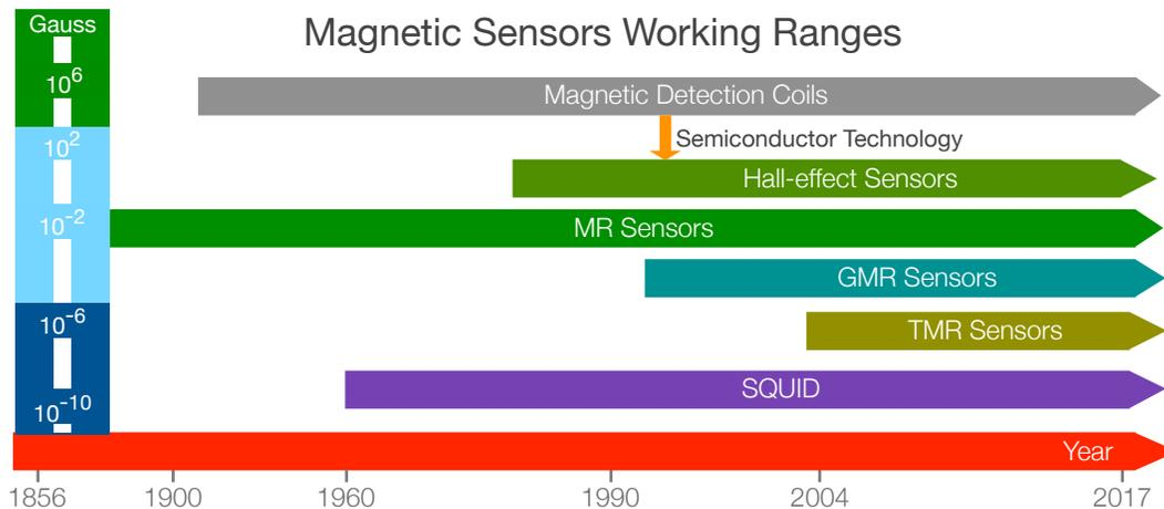
Figure 7. Comparison between magnetic sensors working range.
