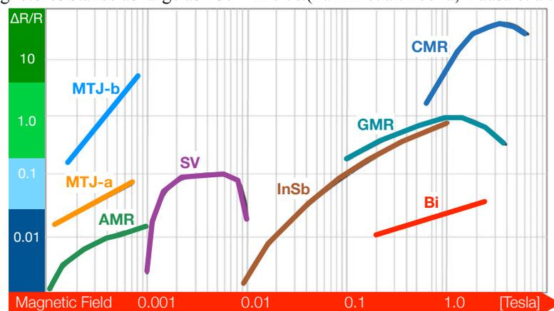
**Figure 6.** Various magnetoresistance effects. Reproduced from (Tumanski 2001, 2016).
