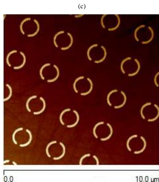
Figure 1 (a): Schematic of an A-SRR with diameter d ; gap angle, \theta = 26^\circ and strip width, w = 100 nm (diagram drawn not to scale). (b) The transmittance spectral response of the 1230 nm diameter A-SRR with that of the simulated data. (c) The atomic force microscope (AFM) image of an array of A-SRRs.
