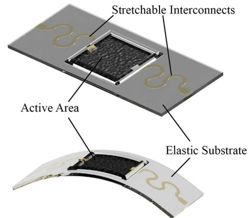
Figure 1: Schematic of the stretchable pH sensing patch with hybrid packaging that can be conformably attached to unconventional surface.
