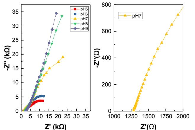
Figure 3: EIS spectrum of fabricated pH sensing patch corresponding to each pH values (left) and magnified image in high frequency range from EIS spectrum for pH 7 (right).
