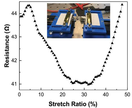
Figure 5: Electromechanical characterization on the stretchable pH sensing patch.
