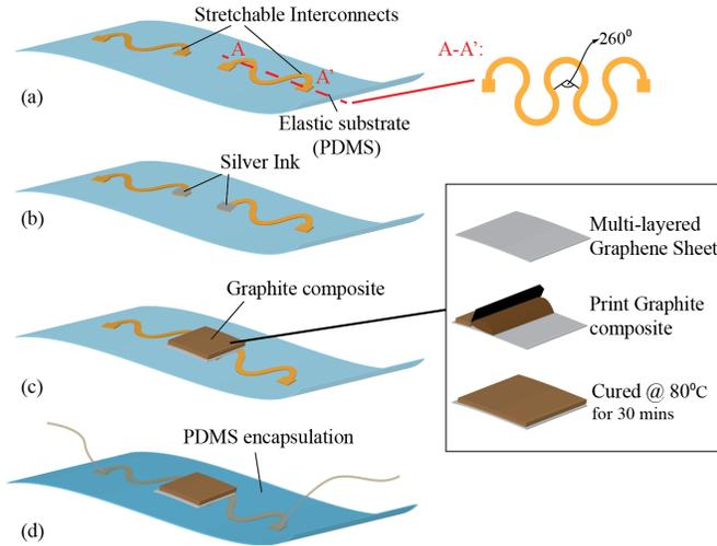
Figure 2: The assembly steps of prototype device including (a) transferring prepared stretchable interconnects to PDMS substrate, (b) applying silver inks on the contact electrode, (c) transferring pH sensing electrode and (d) final encapsulating with electrical wirings.
