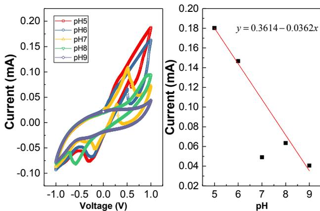
Figure 4: The cyclic voltammetry sweep for the fabricated pH sensing patch. (left) and the pH sensitivity of fabricated patch with the linear fitting. (right).
