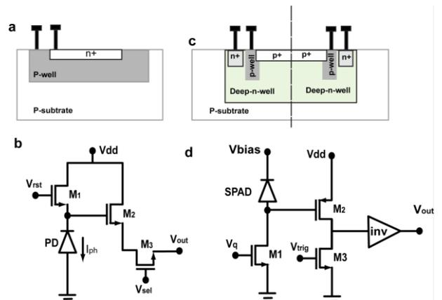
Fig. 1. a) Cross section of a rectangular shaped PD. b) Circuit diagram of a PD pixel. c) Cross section of a circular shaped SPAD. d) Circuit diagram of a SPAD readout. Both detectors were fabricated in a CMOS process.
