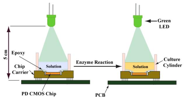
Fig. 3. A schematic illustration of the experimental mechanism of colorimetric sensing. During reaction the solution changes colour, resulting in fewer photons from the LED reaching the photodiode, changing the reading of the PD which indicates the cholesterol level.
