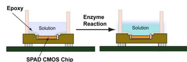
Fig. 5. A schematic illustration of the experimental mechanism of the chemiluminescence detection. The photon emission of the peroxidase conjugated antibodies reaction is detected by the SPAD.
