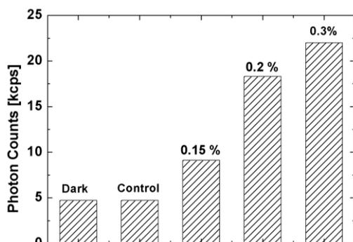
Fig. 6. Varying concentrations of hydrogen peroxide with luminol during a chemiluminescent assay are detected by the SPAD.
