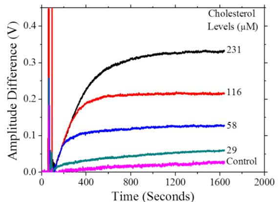
Fig. 4. Experimental results of colorimetric experiments using PD. The measurements show different cholesterol concentrations. The voltage response of the PD increases proportionally to the change in cholesterol concentration.
