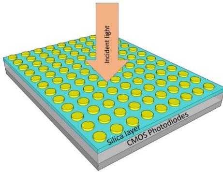
Fig. 7. Schematic of the gold nanodisc array monolithically integrated with CMOS PDs.
