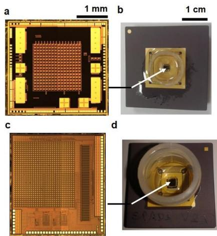
Fig. 2. a) Photograph of the 3.4 mm × 3.6 mm PD array chip. b) Packaged PD chip with epoxy and protection for wet biochemistry. c) Photograph of the 3.7 mm × 3.7 mm SPAD array chip. d) Packaged SPAD chip.
