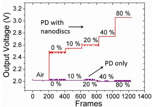
Fig. 8. Change in output voltage of the CMOS PDs with and without gold nanodiscs due to refractive index changes corresponding to different concentrations of glycerol.
