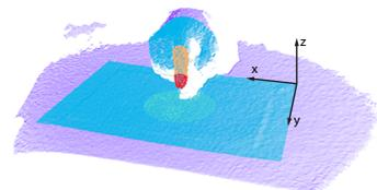
**Figure 2.** Segmented sensor image with points within the interactive surface (blue), the ROI plane (cyan), the detected fingers (yellow) and the user pointer (red).
