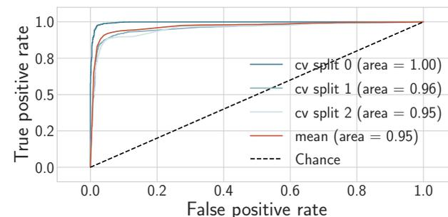
**Figure 3.** Performance of the fingertip touch classification with 3-fold cross validation. Each split trains on two finger types (among three) and validates against the remaining one.
