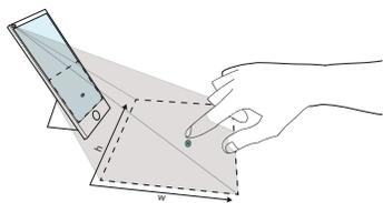
**Figure 1.** Potential interaction setup. A mobile device whose optical sensor creates an on-demand touch surface offers width and height as free parameters.
