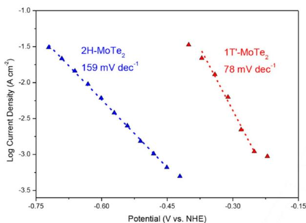
**Figure 4.** Tafel plots of the two polymorphs in 1 M H<sub>2</sub>SO<sub>4</sub>. Plots were obtained as per the conditions described in the Experimental Section, and the current density was recorded after each potential had been applied for 5 min. The dashed lines are provided as a guide to the eye. All current densities have been corrected for resistance.
