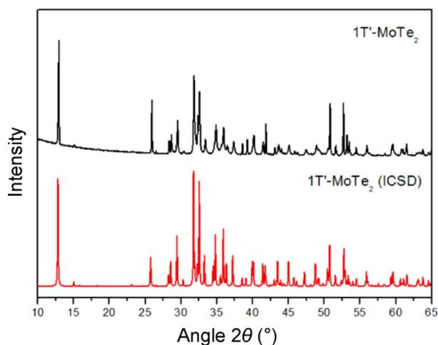
**Figure 1.** Powder X-ray diffraction pattern of 1T'-MoTe<sub>2</sub> (top) and a simulated diffraction pattern from the ICSD database (bottom).<sup>[25]</sup>
