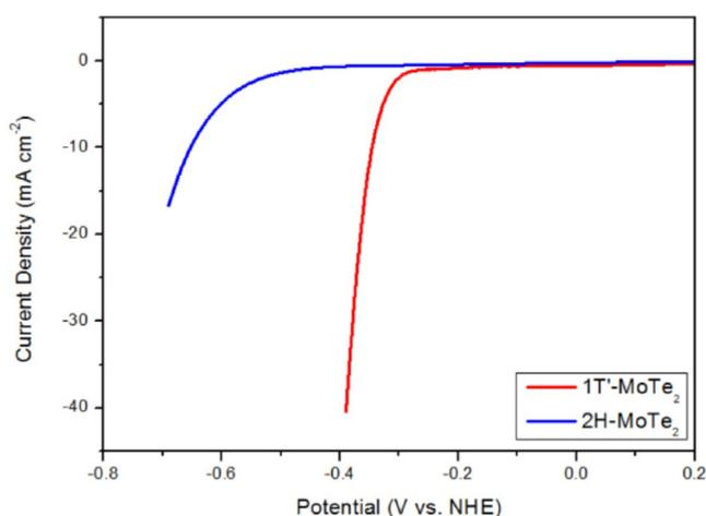
**Figure 3.** Comparison of the current densities achieved by each catalyst in 1 M H<sub>2</sub>SO<sub>4</sub> electrolyte. Catalysts were prepared on a glassy carbon working electrode as described in the Experimental Section. A 3 M Ag/AgCl reference electrode and Pt wire counter electrode were used. Curves were obtained using linear sweep voltammetry at a scan rate of 2 mV s<sup>-1</sup>.
