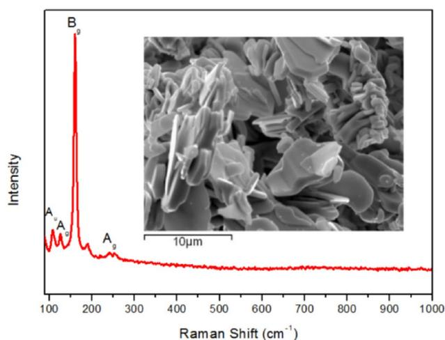
**Figure 2.** Wide-range Raman spectrum of 1T'-MoTe<sub>2</sub> with four major vibrational modes highlighted. The inset shows particle morphology from SEM images.
