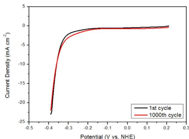
**Figure 5.** Stability test of 1T'-MoTe<sub>2</sub> in 1 M H<sub>2</sub>SO<sub>4</sub> electrolyte obtained by the continuous sweeping of the applied potentials for 1000 cycles using cyclic voltammetry.
