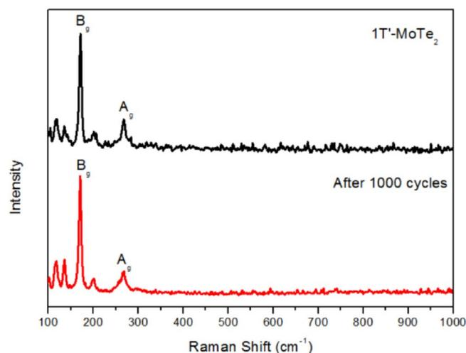
**Figure 6.** Comparison of the Raman spectra of 1T'-MoTe<sub>2</sub> obtained before and after stability tests.
