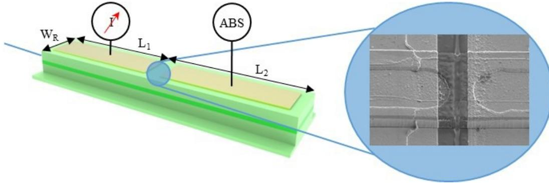
Figure 4. Schematic of GaN device after FIB milling of the top contact
