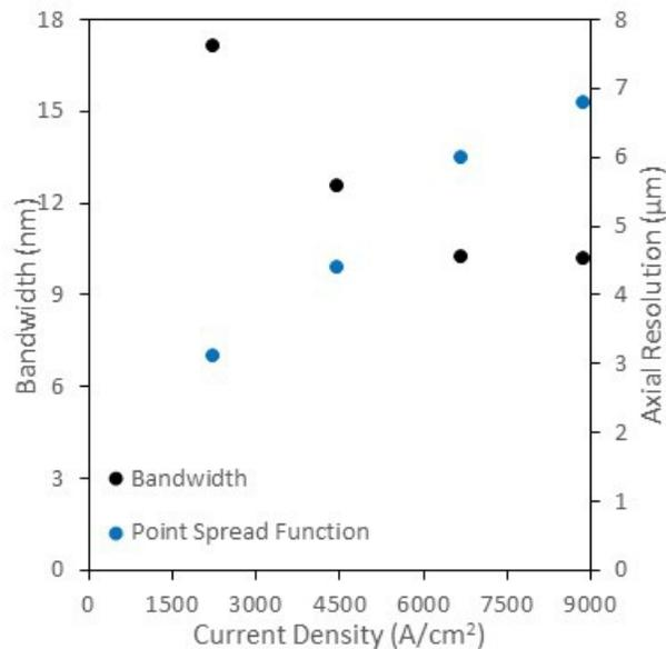
Figure 7. GaN SLED optical bandwidth and resulting estimated axial resolution of the OCT system after FIB milling
