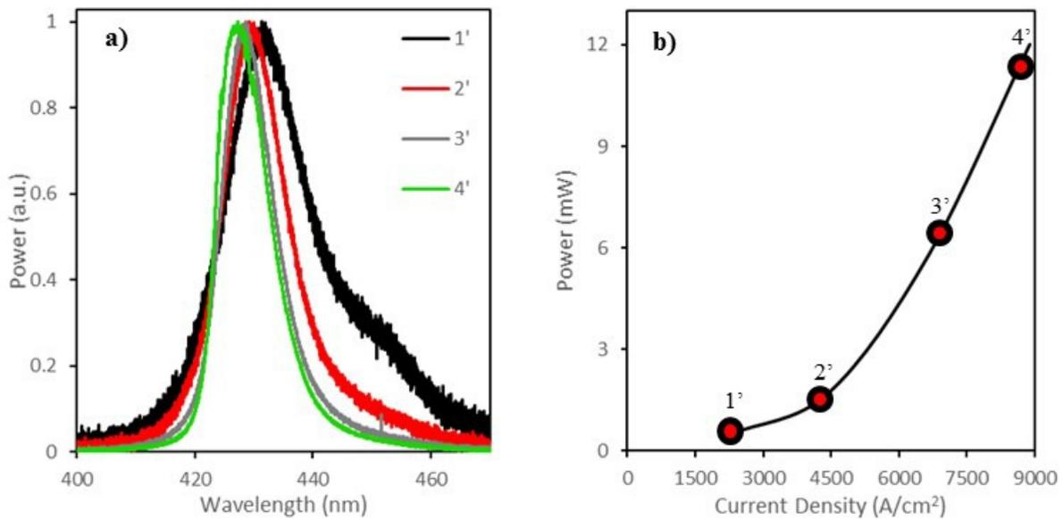
Figure 5. GaN device after FIB milling of the top contact a) emission spectra, b) LI curve
