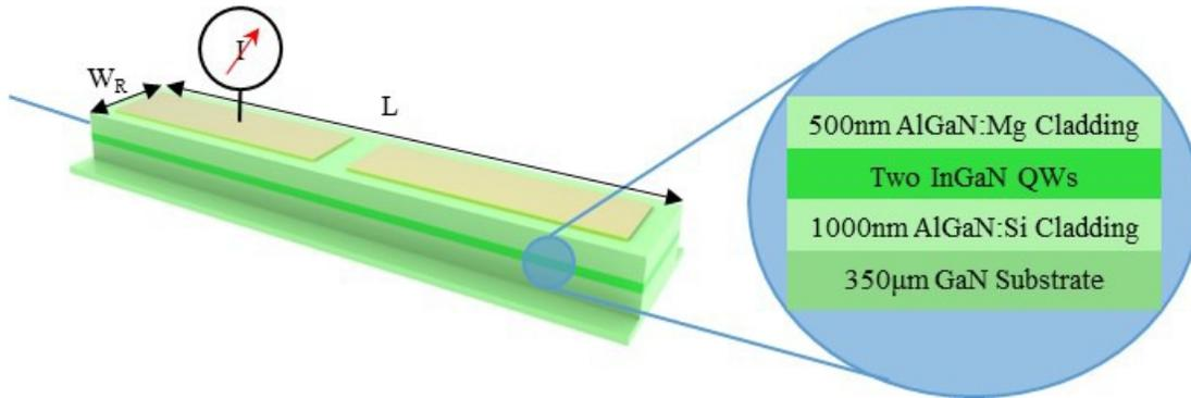
Figure 2. Schematic of GaN device
