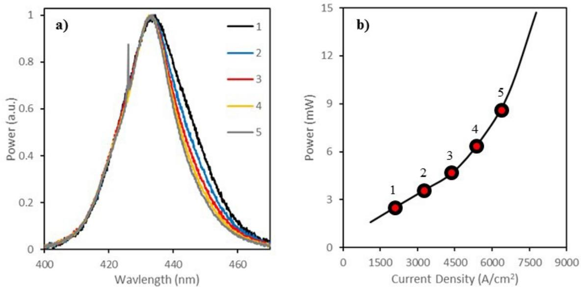
Figure 3. GaN device a) emission spectra, b) LI curve
