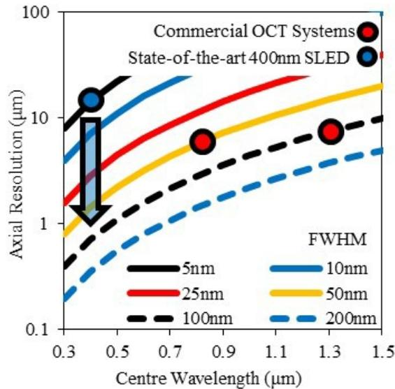
Figure 1. Axial resolution for OCT systems as a function of spectral-bandwidth and central wavelength
