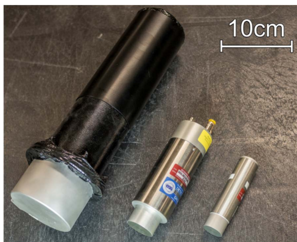
Fig. 1. The detectors employed for the measurements presented in this paper. From the left: NE-213 liquid-scintillator neutron and gamma-ray detector; CeBr 3 gamma-ray spectroscopy detector; YAP(Ce) gamma-ray trigger detector.
