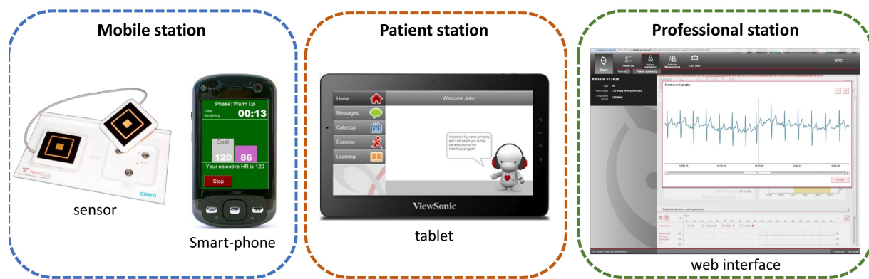
Figure 1. The GEx system comprising the Mobile station (sensor and smart-phone), the Patient station and the Professional station with its web interface
