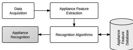
Fig. 2: NILM flow diagram for Load Identification
