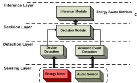
Fig. 1: Multi-Layer Decision Framework for Smart Sensing
