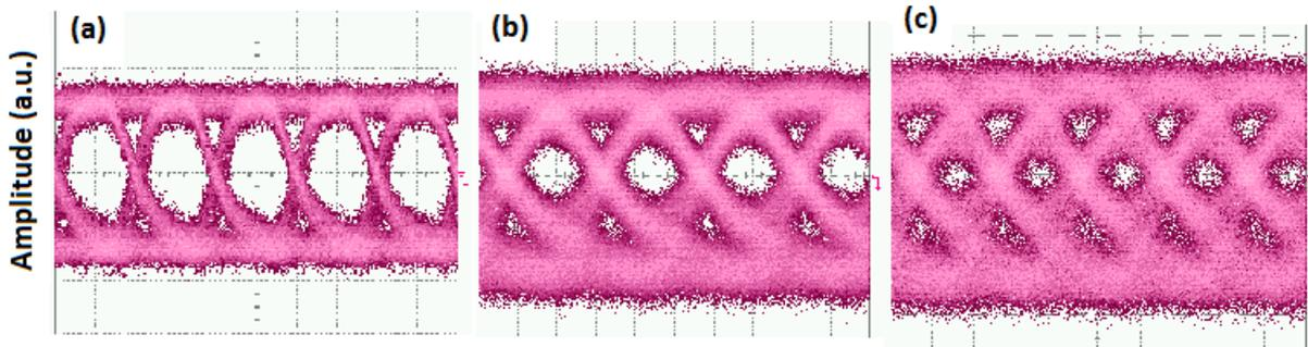
Figure 2. Eye diagrams showing data transmission for a signal transmitted through the water at (a) 1 Gbit/s at 125 mA laser drive current, (b) 2 Gbit/s at 132 mA and (c) 2.488 Gbit/s at 132 mA [4].
