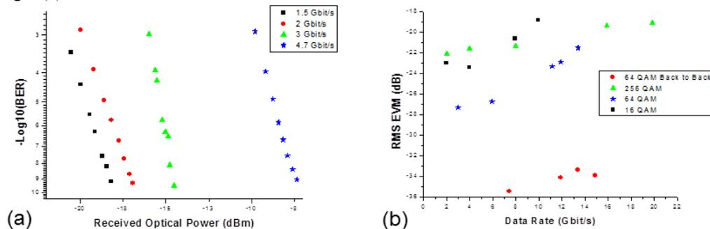
Figure 1: (a) BERs vs. received optical power at 1.5, 2, 3 and 4.7 Gbit/s at optimum bias currents for each bit rate; (b) RMS EVM magnitude at 256QAM, 64QAM and 16QAM. 64QAM back to back shows instrument noise.
