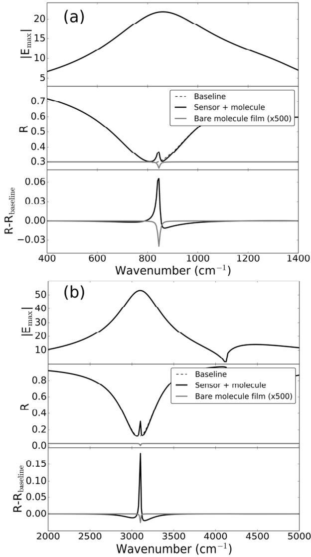
**Fig. 2.** (a) Local field enhancement and typical SEIRA signal for a Ge sensing platform operating at  $845 \text{ cm}^{-1}$ . (b) Local field enhancement and typical SEIRA signal for a Au sensing platform operating at  $3100 \text{ cm}^{-1}$ .
