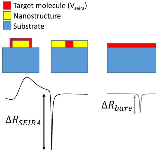
**Fig. 1.** Schematic representation of nanoantenna and nanoslit SEIRA sensing platform and corresponding baseline corrected reflectance SEIRA signal ( $\Delta R_{SEIRA}$ ), along with the reference reflectance signal for the same volume  $V_{SEIRA}$  of target molecules deposited on the bare substrate ( $\Delta R_{bare}$ ).
