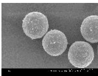
Fig.3: SEM image of silver-coated PMMA microspheres with 700 magnification times.
