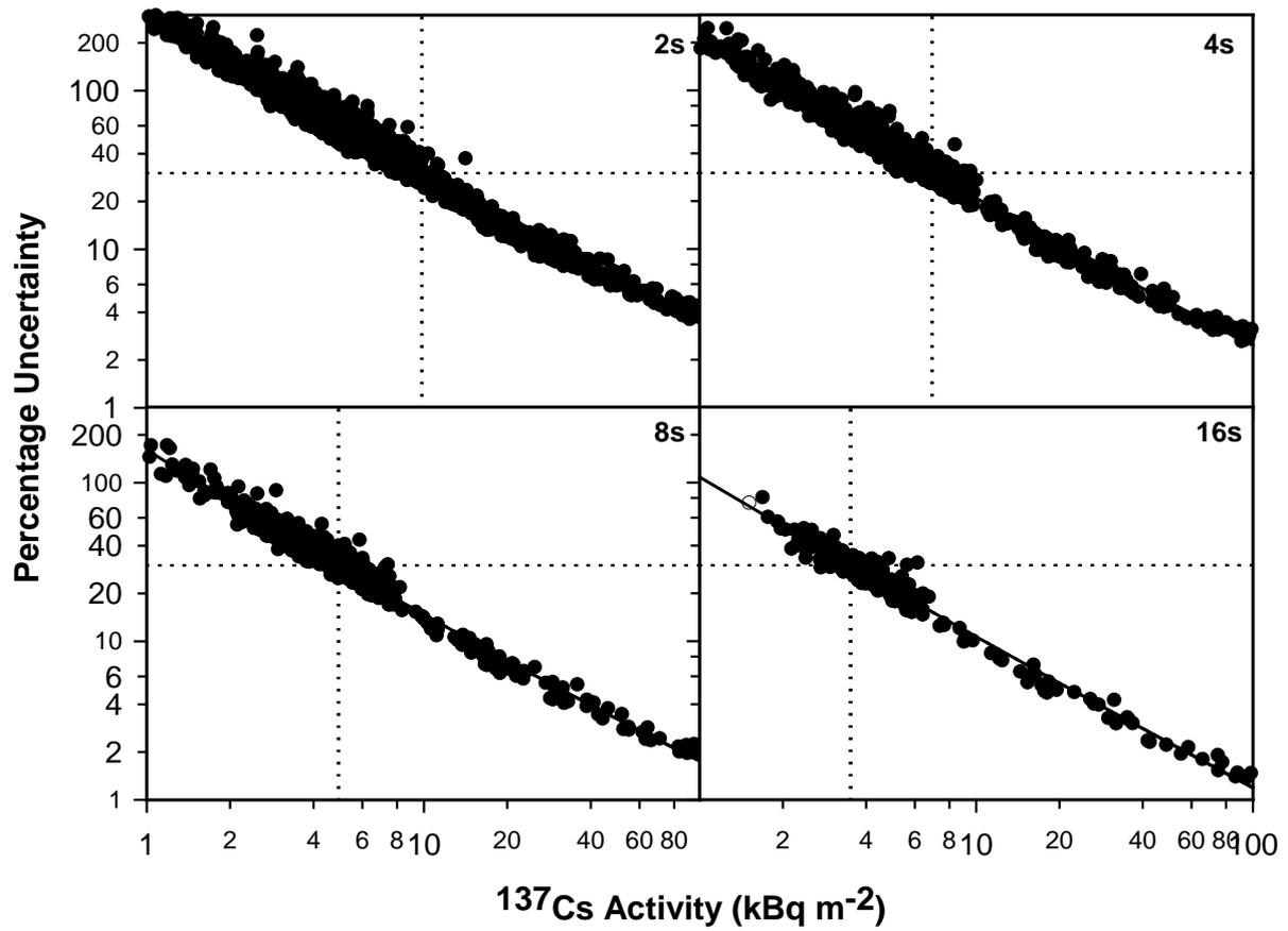
Figure 1: Percentage uncertainties on  $^{137}\text{Cs}$  stripped count rates for 2, 4, 8 and 16 s integration times.
