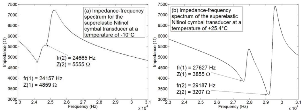
Fig. 2. Impedance-frequency spectra for different material states.
