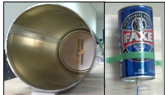
Fig2. Endfire dipole antenna
