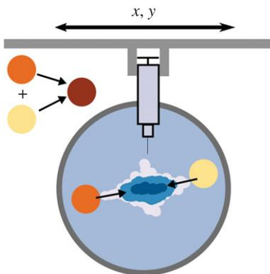
**Figure 6.** The use of the dropletbot to conduct experiments with droplets with different chemistries in a Petri dish where the syringe is adding chemicals to affect the behaviour of the droplets by creating the gradient conditions needed for chemotaxis to occur.
