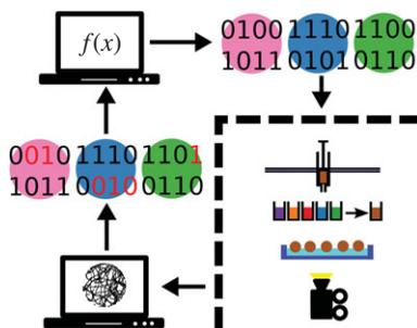
**Figure 3.** A schematic diagram of the robotic platform coupled to an optimization algorithm. A computer (top left) generates a number of input ‘formulations’ (top right), and each formulation is tested as droplets in a Petri dish (bottom right). The behaviour of the droplets is monitored by a camera mounted under the dish and trajectories of the generated droplets are analysed in a computer to generate formulations for the following round of droplet chemistry.
