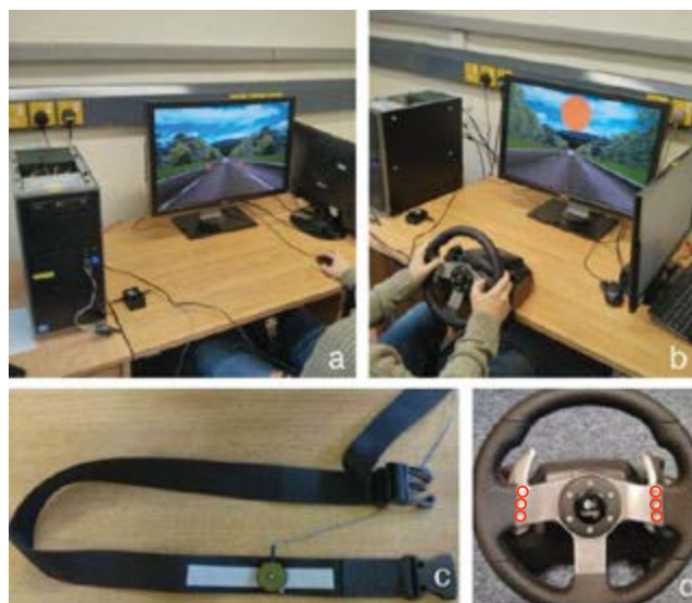
Figure 1. The setup of Experiments 1 (a) and 2 (b), the waist belt with the Tactor (c) and the steering wheel used in Experiment 2, with the response buttons highlighted (d).
